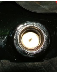
Flow Restrictor fitted grove side down at rod end
