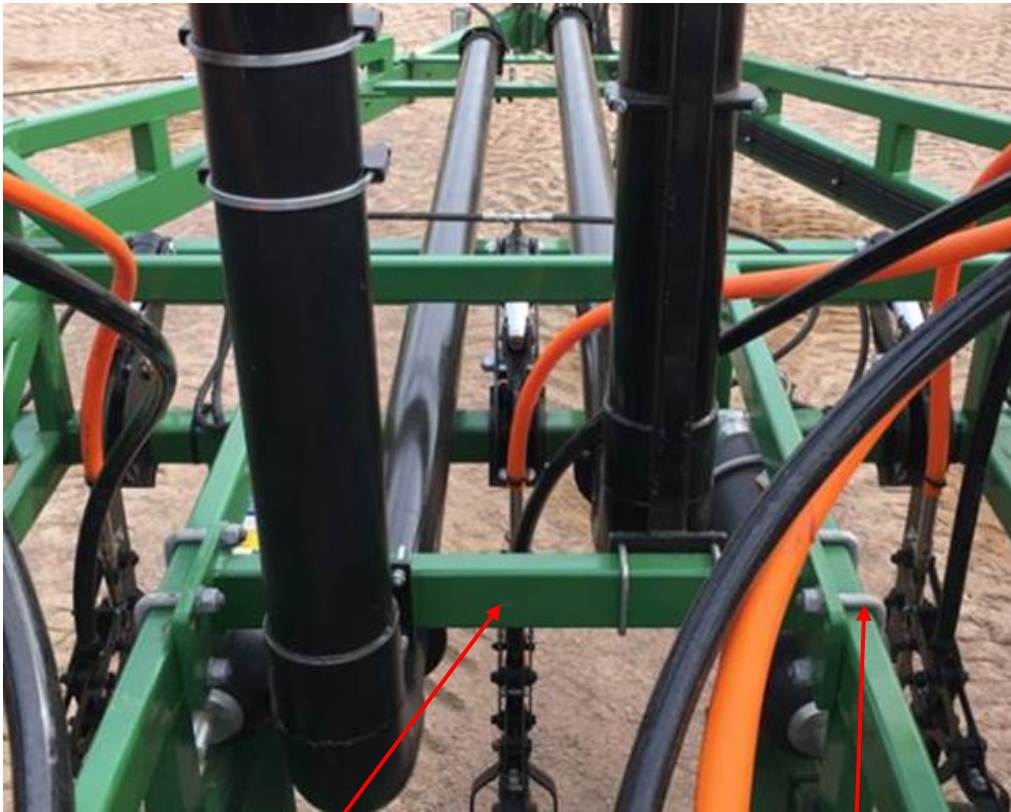
#34586 U Bolt Set M20x102x100mm SS (Replaces 05437) 4 required
