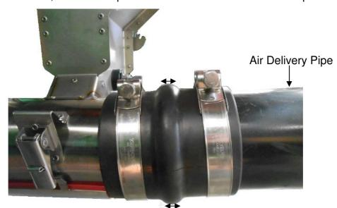
Ausplow recommends trimming the steel air delivery pipe to create a 20mm gap between air pipes to provide proper fitment of the coupler.
