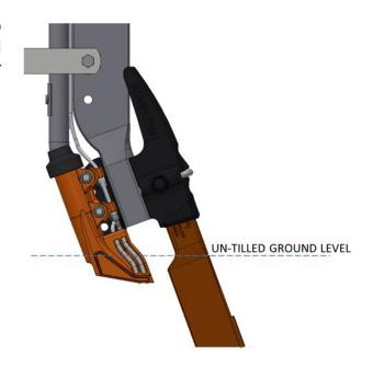
Fitting the fertiliser boot to the tine assemblies will require the 32mm stainless steel fertiliser tubes. The lower fertiliser tube clamp is now removed. The rubber Fertiliser Boot Protection Cap is fitted first to the fertiliser tube prior to attaching the boot.
