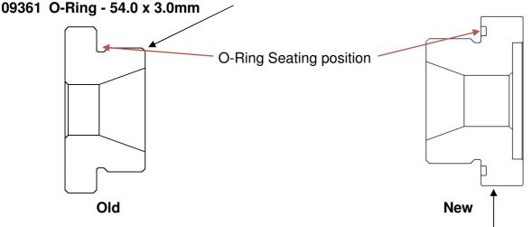
27092 Reducer Bush – Accumulator Adaptor 2" BSPP M O-Ring To ¾" BSPT F 27264 O-ring 70.0 x 3.5mm
