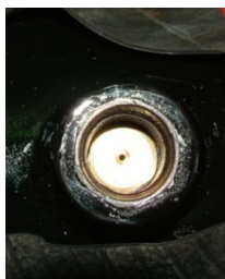
Flow Restrictor fitted groove side down at rod end
