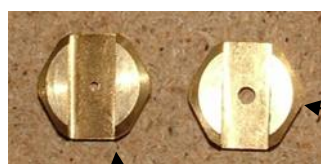
Flow Restrictor fitted groove side down at rod end
