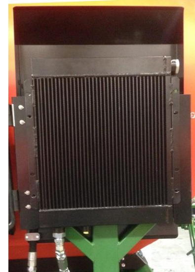
Core size 23 with internal bypass
