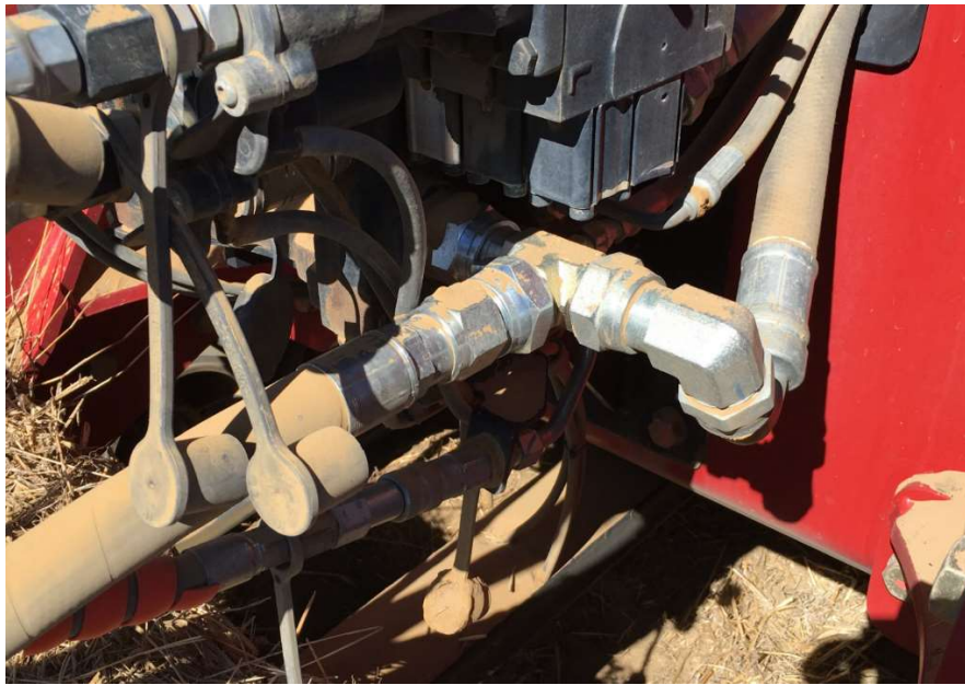
Picture 4.6.1: Return Line Hard Coupled
