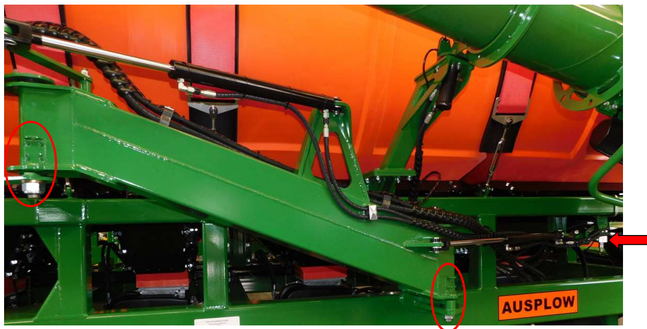
Picture 6.2.5 Auger Arm Cylinder connected to Cylinder Lock Valve
