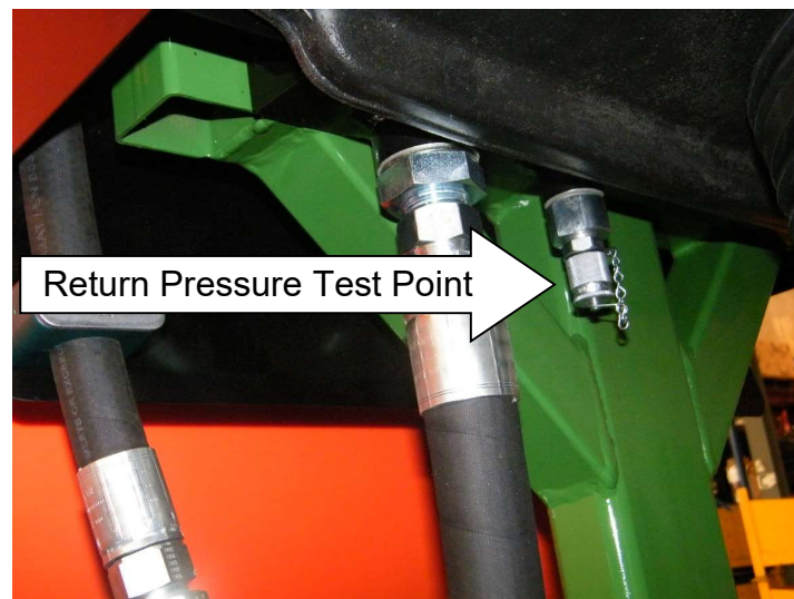
Picture 4.6.2: Return Oil Pressure Test Point
