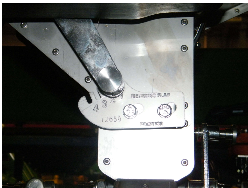
Picture 8.3.5: Metering Flap
