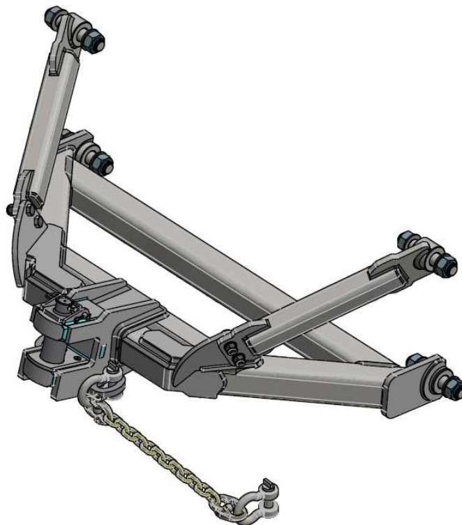
Figure 3.3.3: Rear hitch of the Tow Between Multistream with the safety chain in place through the lug.
