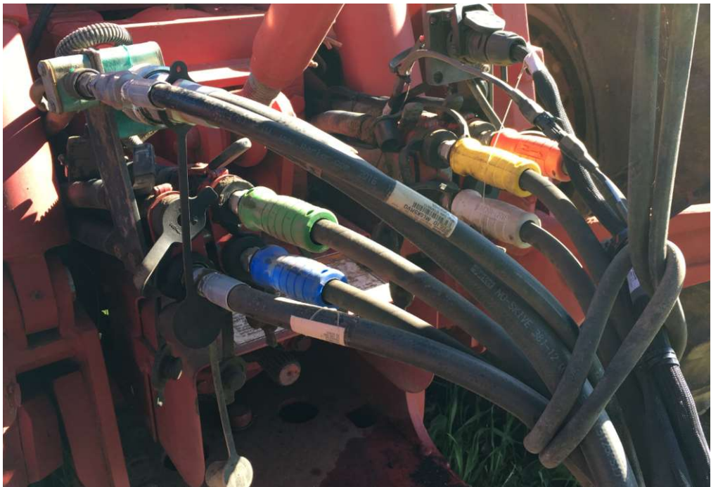
Picture 4.6.3: Hydra Grip Hose connectors
