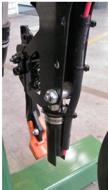
Picture 10.4.2: V4 Tine with Friction Flow Liquid Tube
