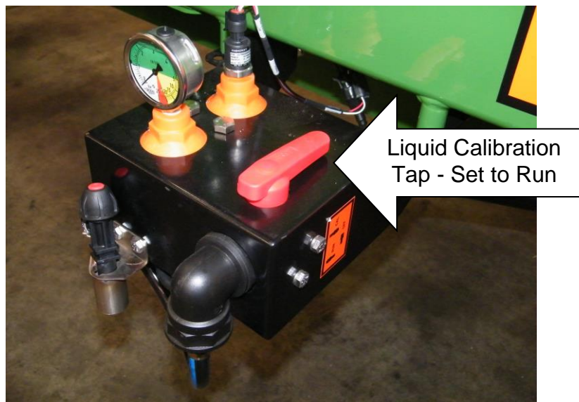
Picture 9.7.5: Liquid Calibration Tap Set to Run
