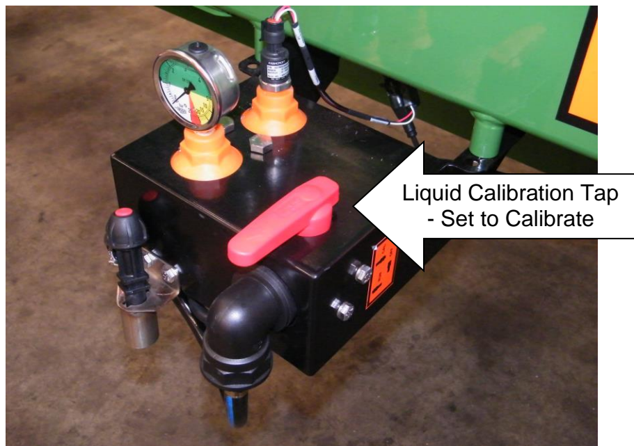
Picture 9.7.3: Liquid Calibration Tap Set to Calibrate
