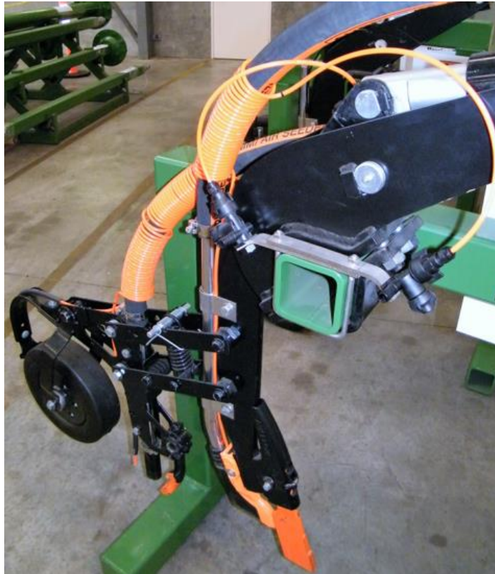
Picture 10.4.1: V4 Tine with Friction Flow Liquid Tube
