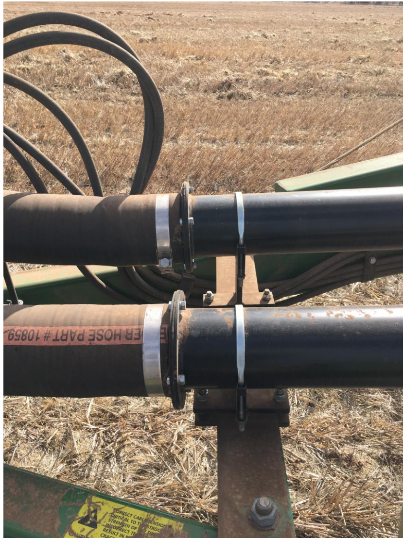
Picture 8.1.2: Air Hose joining to Auseeder – Tow Between Models
