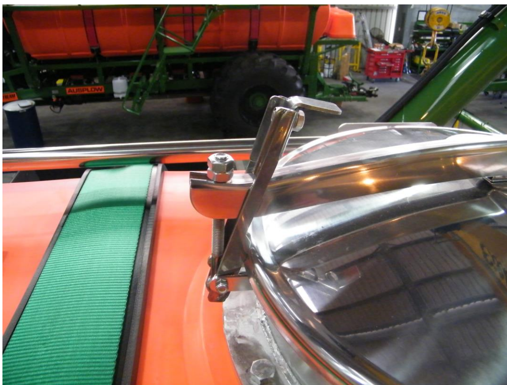
Pictures 11.4.2: Correct Tank Lid Lever Engagement
