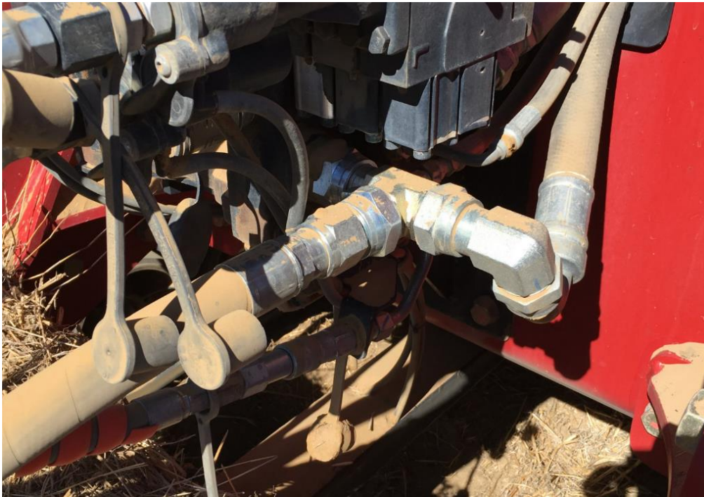
Picture 4.6.1: Return Line Hard Coupled
