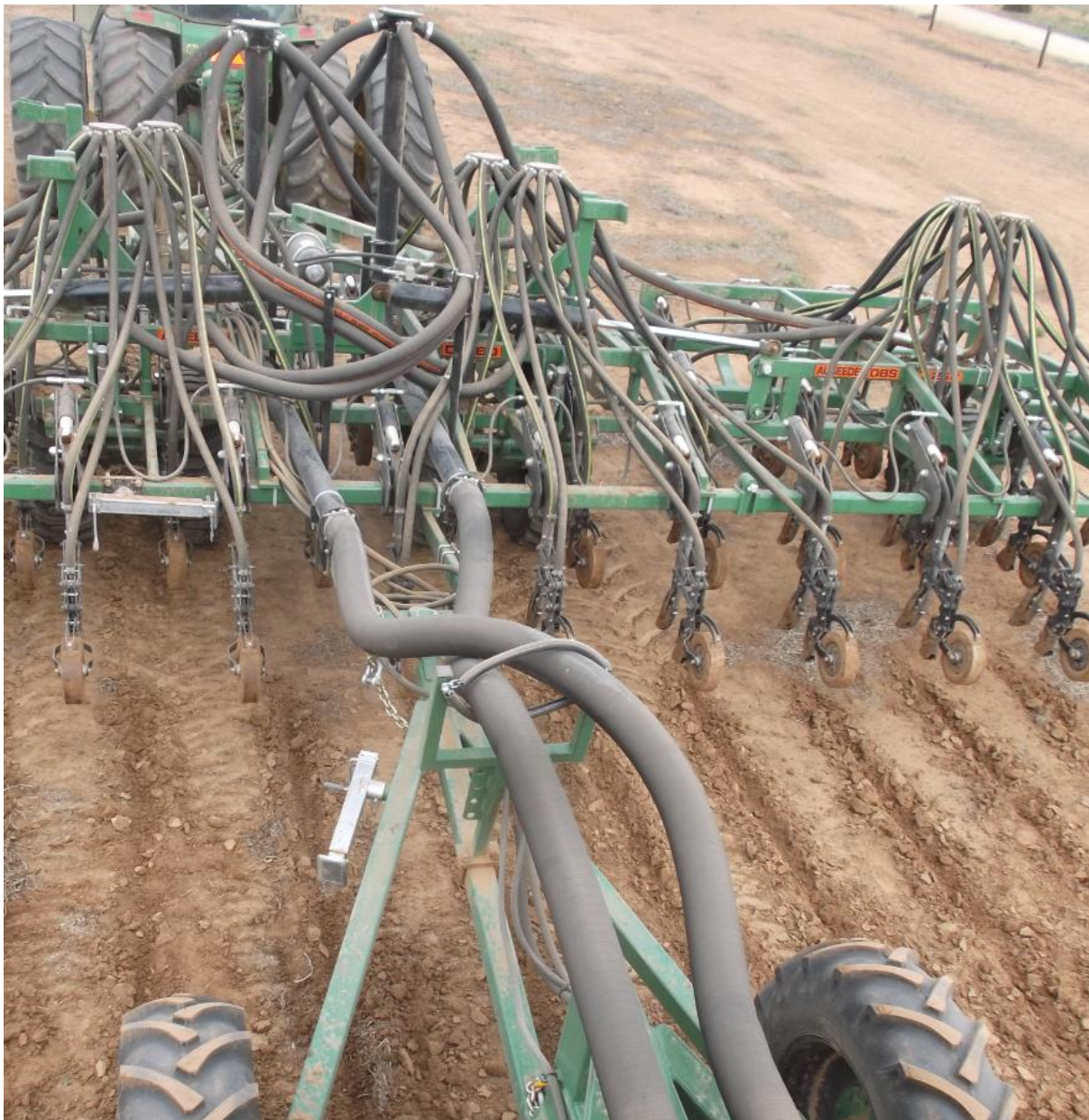
Picture 8.2.1: Side by Side Primary 5" Hose – Tow Behind
