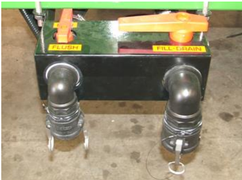
Picture 10.5.2: Fill Station – Liquid Equipped Multistream Tanks
