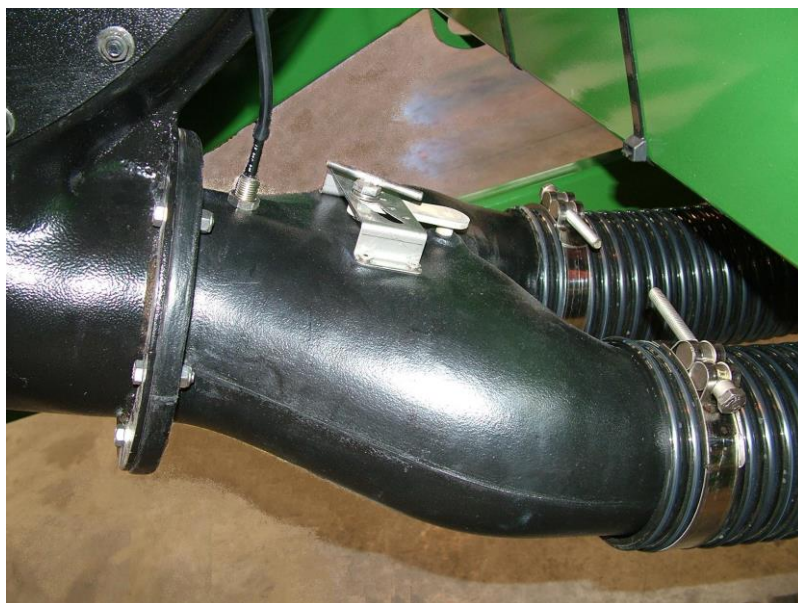
Picture 9.6.1: Air Dividing Flap
