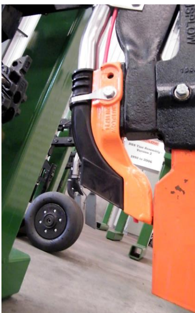
Picture 10.4.2: V4 Tine with Friction Flow Liquid Tube
