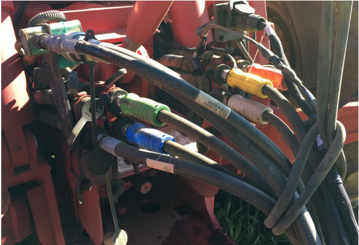
Picture 4.6.3: Hydra Grip Hose connectors
