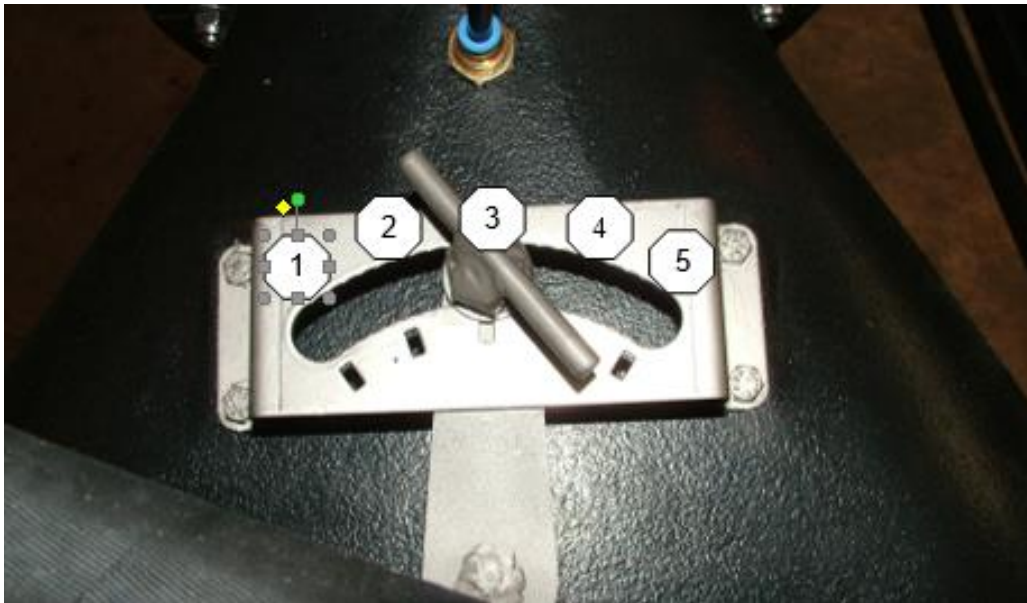
Picture 9.6.3: Air Flap Position 3 – Equal Airflow to Both Air Pipes (All)
