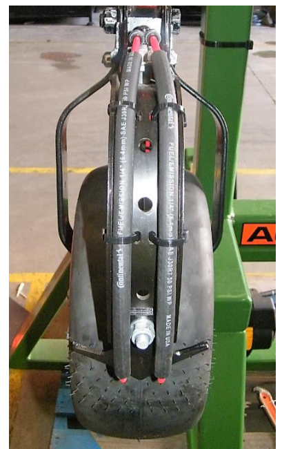
Picture 10.4.2: V4 Tine with Friction Flow Liquid Tube
